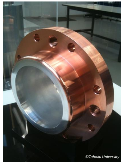
Thick deposit of copper (between 50 to 60 mm) obtained by "Cold spray." The deposited copper is machinable: holes for screws, flanges, etc. © Tohoku University
